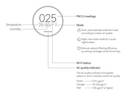
Note: the air purifier automatically adjusts the display brightness based on ambient light.
